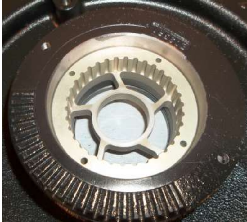
Radial shredder ring installed.
