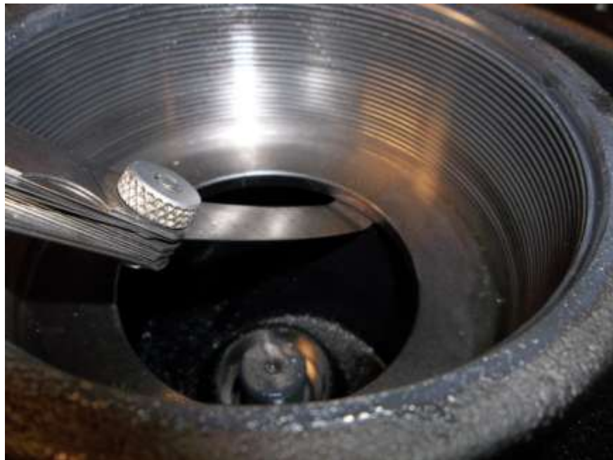
Feeler gauge shown between impeller vane and top of suction cover.
