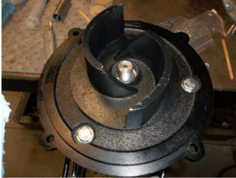
Impeller shown on shaft. Note volute case has not been added to give clearer picture of the impeller on the shaft.
